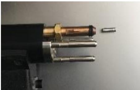
〈Step 1〉 Set CD weld gun in the CD stud welding machine...
