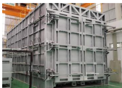
4 meter(W) x 4 meter (H)x 10 meter(D) Large ovens suitably designed to process large equipment
