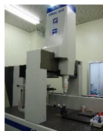
3-D Coordinate Measuring Machine
